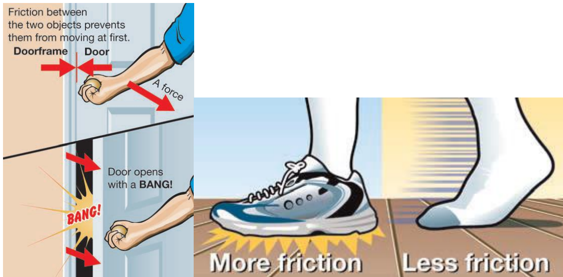
Figure 12.3: A stuck door is an example of stick-slip motion.
